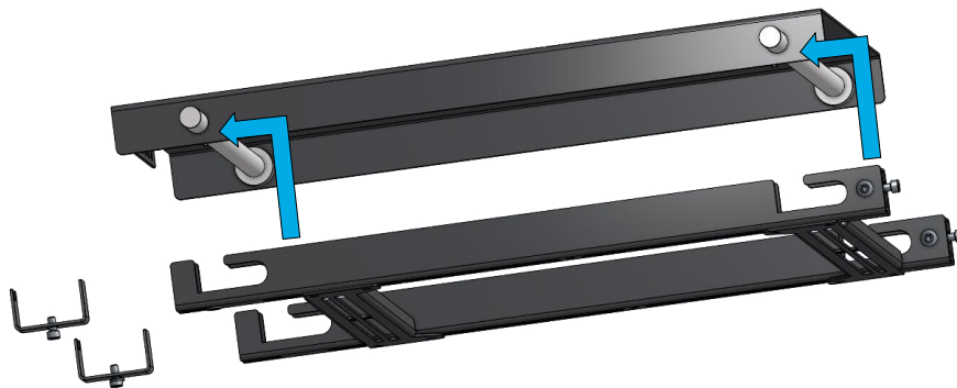
Fig.5. Mount Plate with projector alignment - step 1
